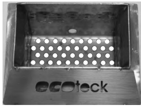
Clean basket with all the holes clearly visible
